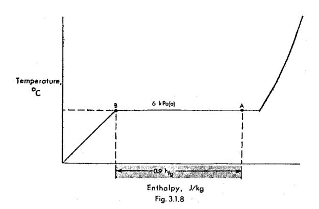
The steam enters the condenser at point A where it has already lost 10% of its latent heat. The condensate leaves the condenser at point B where it is saturated liquid. The change in enthalpy is the remaining latent heat, ie, 0.9  $h_{fg}$  at 6 kPa(a).
